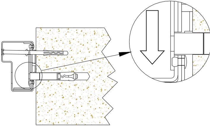
**12.** Unscrew and remove the cap head screw, leaving the frame fixing in the wall. Working through the frame access hole, move the sliding washer plate across, so that its 10.5mm hole is concentric with the 16mm frame tray hole.
