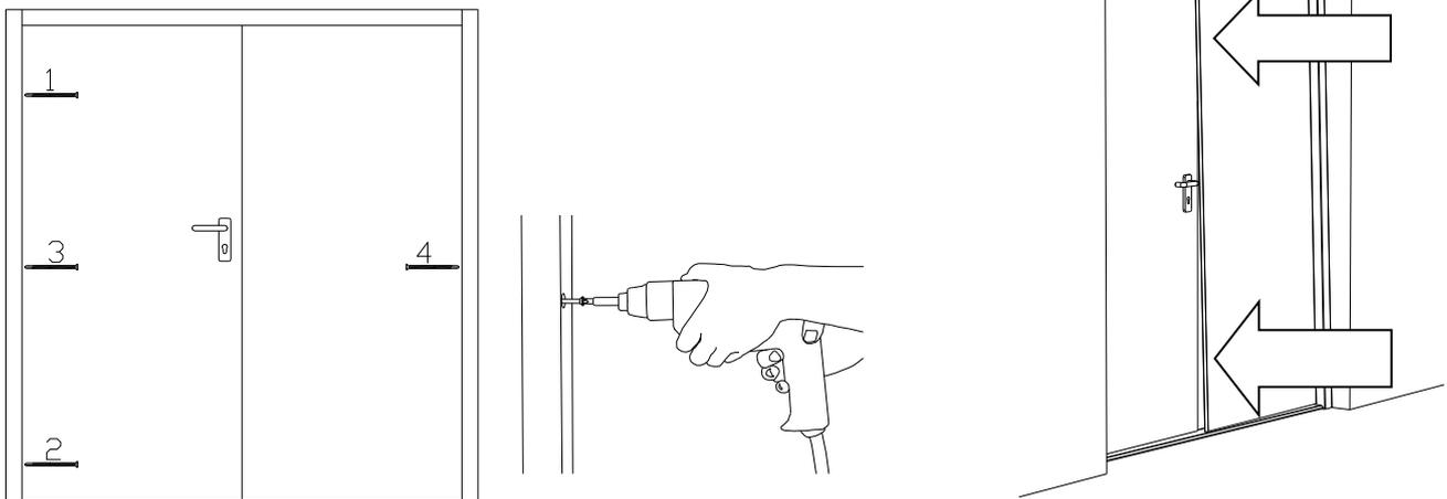
**6.** Using long countersunk frame fixings, first fix as shown, with 3 fixings in the active leaf jamb and 1 in the fixed leaf jamb.
