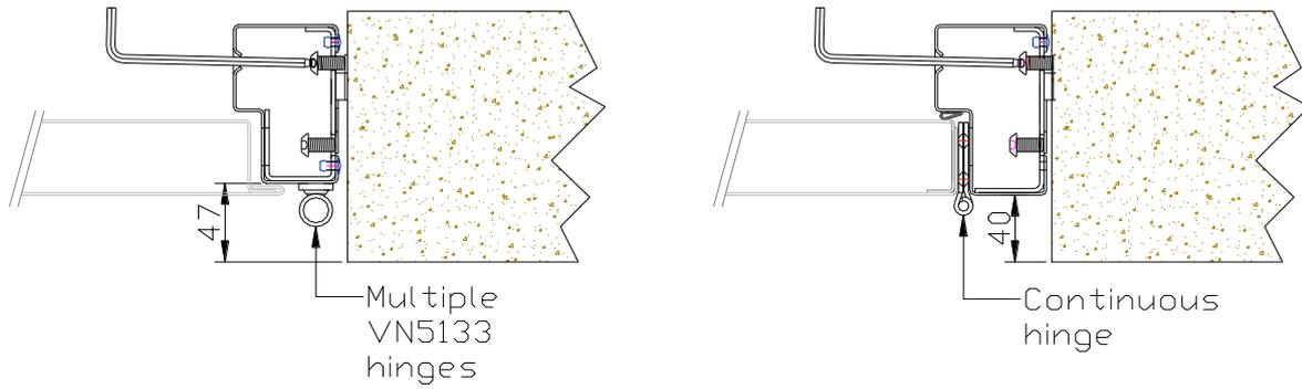
**5.** To avoid the fixings breaking out of the wall later, set the jambs back these minimum distances for the relevant hinge type fitted:
