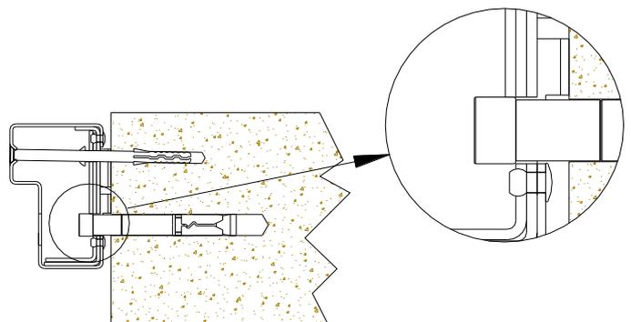
**11.** Insert the fixing as shown, so that the underside of the cap head screw butts up to the inside of the frame tray and does not cover the sliding washer plate. Partially tighten the screw, so that the fixing starts expanding and grips the concrete.
