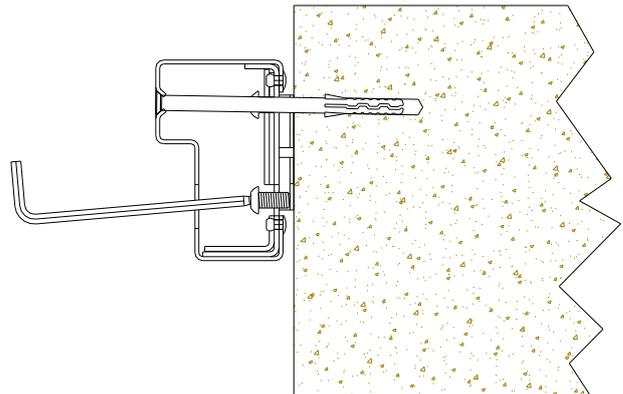
**9.** Open the door fully, then tighten the frame adjusters in the reveals. Using the 5mm Allen key, tighten the frame adjusters until the ends of the spreader plates are flat against the wall.
