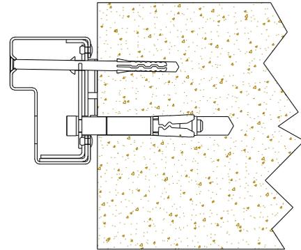
**13.** Refit the 10mm cap head screw and tighten fully.
