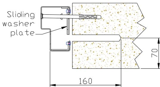
**10.** Ensuring that the sliding washer plate is away from, and not covering the 16mm frame tray holes, drill through the access holes in face 2 with a 15mm masonry bit to a depth of 160mm.
