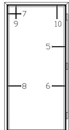
**6.** With the door nearly closed, check the alignment between the lock edge of the door and the frame seal, at both the top and the bottom of the door.
