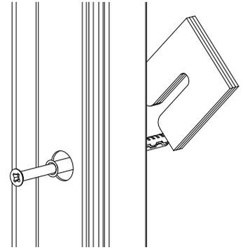
**5a.** First fix in the sequence shown, with 2 fixings in the hinge jamb and 1 in the lock jamb.
