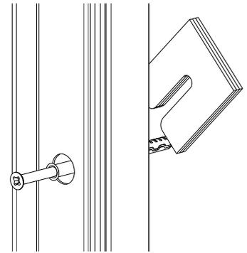
**5a.** First fix in the sequence shown, with 2 fixings in the fixed leaf jamb and 1 in the active leaf jamb.
