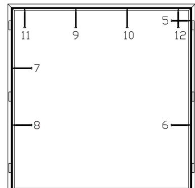
**6.** Close and bolt the fixed leaf, then with the active leaf nearly closed, check the alignment between the meeting stiles for an even seal gap, at both the top and bottom of the doors.
