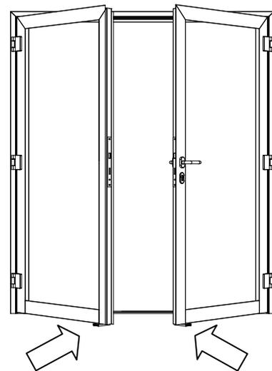
**4.** Open both doors carefully to approx. 45°, taking care not to disturb the frame, then temporarily pack the lock edges of the door leaves off the floor, keeping the jambs vertical.
