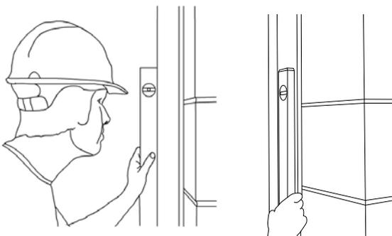
**3.** Ensure that the frame is vertical in both planes, particularly the fixed leafs hinge jamb, and that the top of the doors are still aligned.
