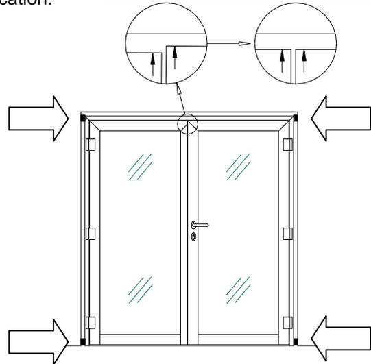
**2.** Align and wedge the frame into the opening, using temporary packers at the corners.
